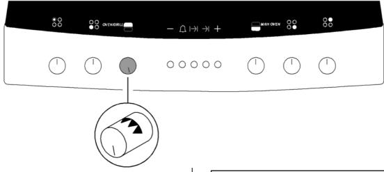
To operate the grill turn the top oven/grill control clockwise to the full power setting (▼▼▼), then turn down as necessary.
